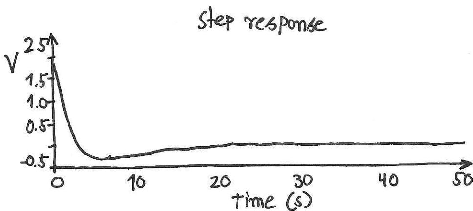
The highpass filter attenuates low frequencies, so the DC-part of the step is not visible on the output.
